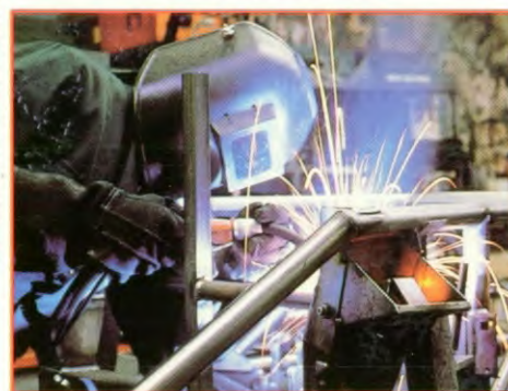
JIG WELDING THE CHASSIS
