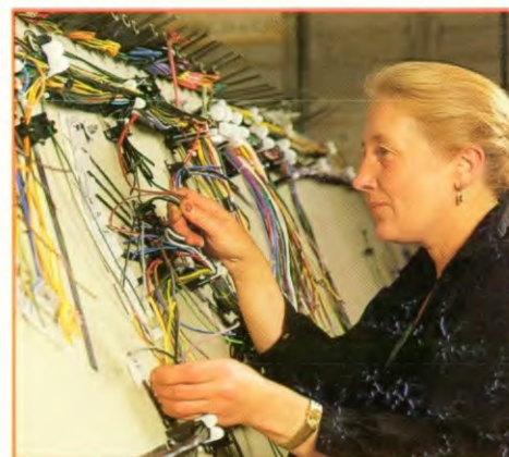
WIRING LOOM CONSTRUCTION
