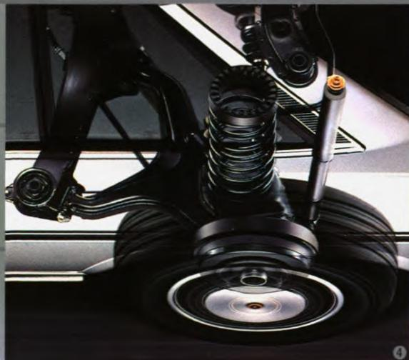
*Cressida performs! Super-responsive engines are now more powerful than ever, and Cressida combines this power with advances in handling and aerodynamics. Cressida offers three engines to choose from, including a highly-refined 2.0-litre super-responsive gasoline engine with a broad power band and excellent acceleration. Independent suspension, with MacPherson struts in front and semi-trailing arms in the rear, gives you extraordinary handling and control, while rack and pinion steering*
