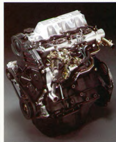
2.0-liter diesel 54 kW/4700 tpm. 132 Nm/3000 tpm.
