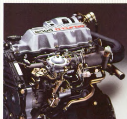
2.0 Turbo Diesel 2C-T 62 kW/4500 tpm 164 Nm/2400 tpm
