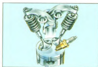
Klepbediening 1.3 liter motor
