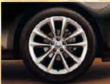
5 Lichtmetalen velg, 7,5 J x 18 en 8 J x 18, multi-spoke design, bandenmaat 225/45 R 18 of 235/45 R 18 (PZW/PZK).
