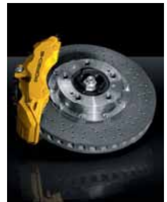
Porsche Ceramic Composite Brake (PCCB)
