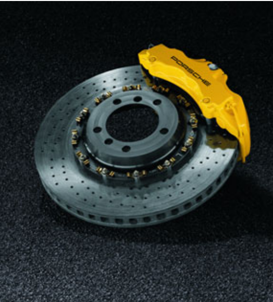
Porsche Ceramic Composite Brake (PCCB)
