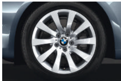
Lichtmetalen BMW wielen in turbinestyling 271 , 8 J x 18 inch, bandenmaat 245/50 R 18 Y.
