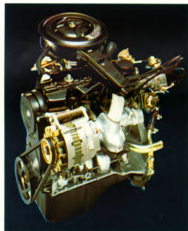
Lichte 4-cilinder 1 liter motor.
