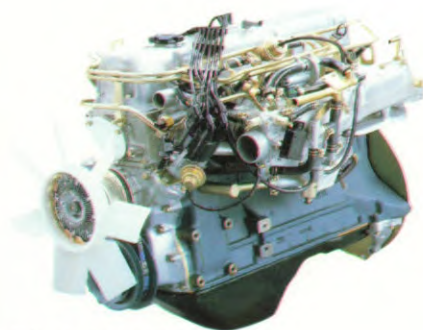
6 Cilinder, 2.4 liter benzine.
