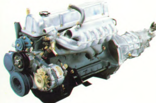
6 Cilinder, 2.8 liter Diesel.
