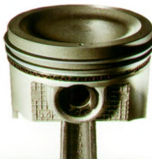
Specially designed piston with additional cooling channels.
