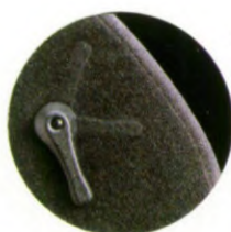
Driver's seat features an adjustable lumbar support lever.
