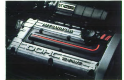
2.0 liter 16V DOHC ECI-Multi-Point benzine motor
