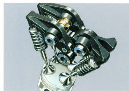
4-valve-per-cylinder engine design ensures optimum breathing efficiency, in turn delivering excellent fuel economy and fewer emissions without compromising on power.
