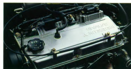
Lightweight and compact, the 2.0-litre 16-valve ECI-MULTI petrol engine's single overhead camshaft design offers smooth, economical performance. Roller rocker arms increase efficiency for higher power, while the highly rigid structural design ensures low noise and vibration levels.
