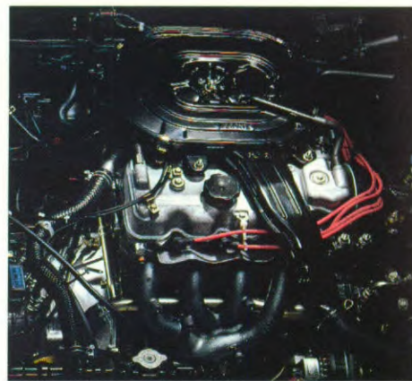
2.0 liter benzinemotor (vermogen 75 kW/6000 rpm)
