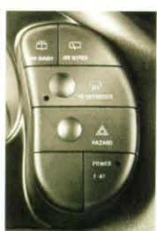
AND TO YOUR RIGHT Cluster at the right of the steering wheel contains controls for rear washer/wiper and defogger. Also located here are switches for hazard flashers and the Power E-AT function which is described in text on this page.
