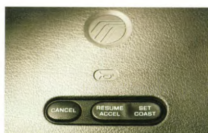
FINGERTIP SPEED CONTROL After activating the speed control with the instrument panel switch, you set the desired speed with these buttons. Note their convenient location near the center of the steering wheel, close to your hands.
