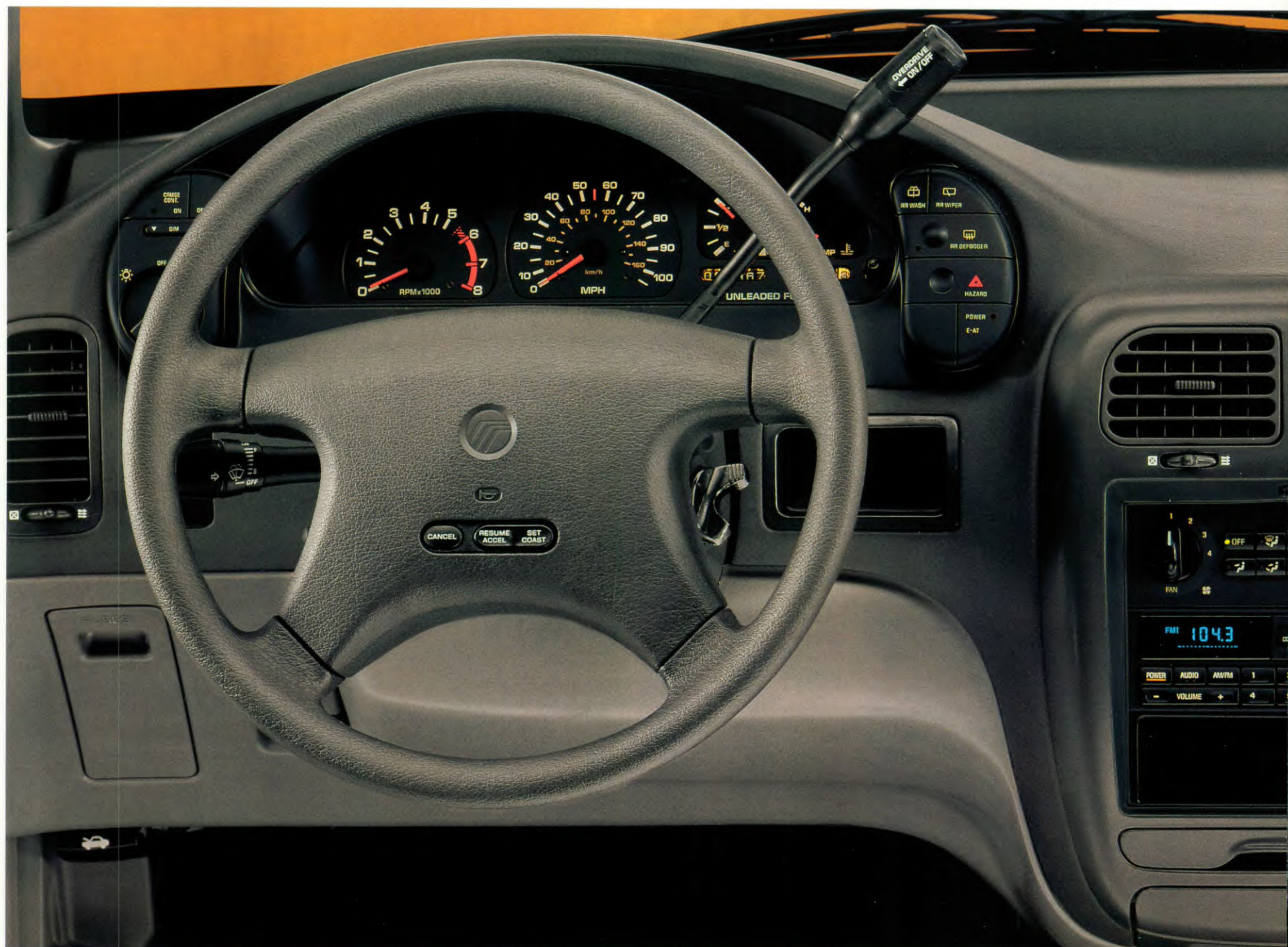
OVERDRIVE LOCKOUT SWITCH Gear selector lever contains a button which permits you to lock out the fourth-speed overdrive transmission function, providing increased engine braking when driving in hilly areas.
