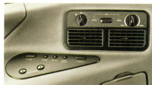
REAR PASSENGER TEMPERATURE AND AUDIO CONTROLS Available remote controls for the heater/air conditioner and audio system permit rear seat passengers to adjust the temperature and select their own entertainment. Master control override remains with the driver.
