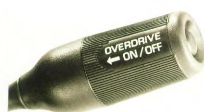
OVERDRIVE LOCKOUT SWITCH Gear selector lever contains a button which permits you to lock out the fourth-speed overdrive transmission function, providing increased engine braking when driving in hilly areas.
