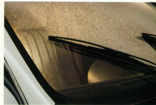
Optional heated Insta-Clear ® windshield defrosts windshield in two minutes or less.
