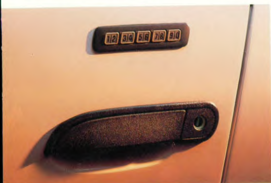
Optional keyless entry unlocks driver's door with simple combination.
