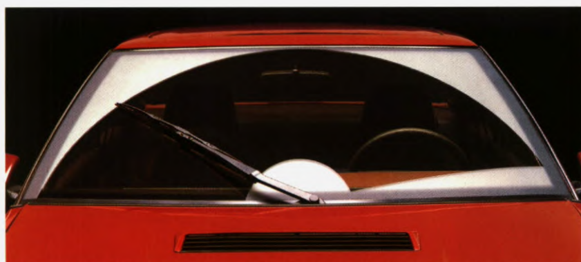
The single-blade wiper reaches up and out on a pivot during its stroke for wide coverage.
