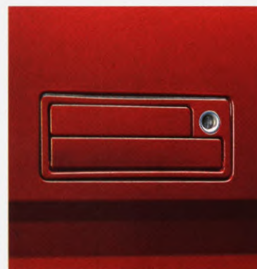
The door handles have aircraft-like flaps to ensure smooth air flow.
