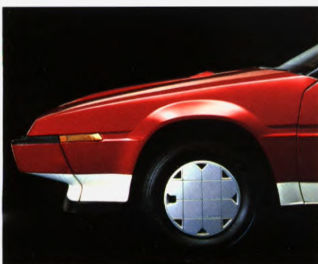
The down-sloping bonnet and front air dam are of an integral construction.
