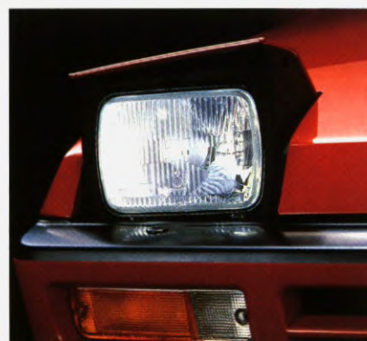
The retractable headlights have good aerodynamic qualities even when they are up and in service.
