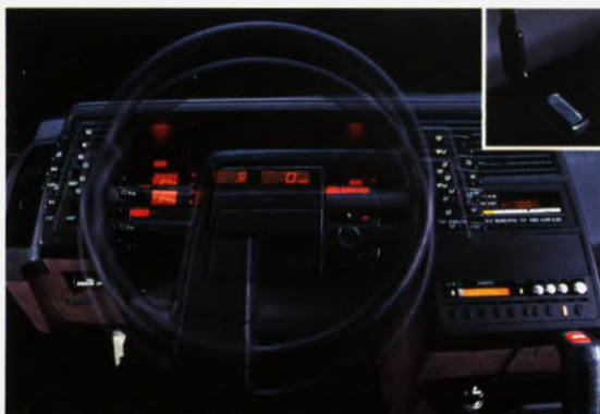
A memory device always returns the tilt steering wheel to the position you preset.
