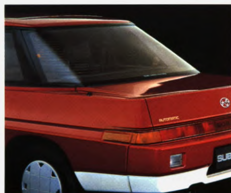
The wrap-around rear window and high-rear deck make positive use of air flow.
