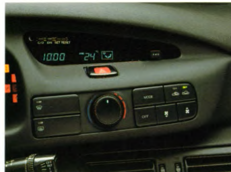
Automatisch geregelde airconditioning.
