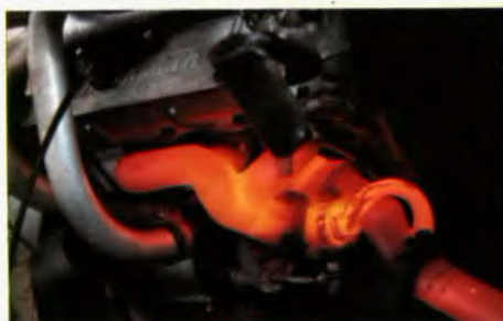
Biturbo engine on the dynamometer during extremely heavy endurance tests at maximum power and speed
