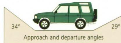
grounded. And it crosses fords with ease, taking water up to half a metre deep in its stride.
