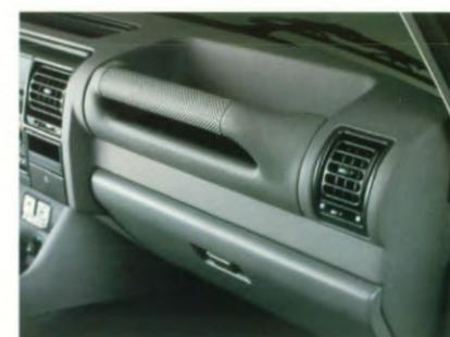
open the lid, you'll find a set of two cup- or glass- holders. Smooth-acting, hydraulically-damped struts slide out another set of holders from under the centre of the fascia, beneath the heating and ventilation controls.
