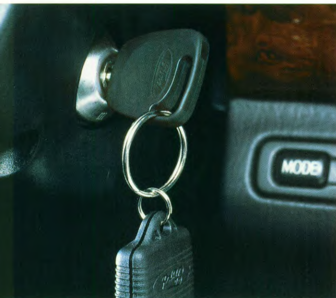
Ford's Passive Anti-diefstal Systeem (PATS).
