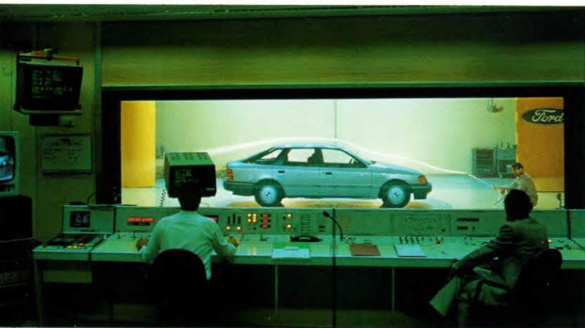
Aerodynamische tests in Ford's windtunnel.
