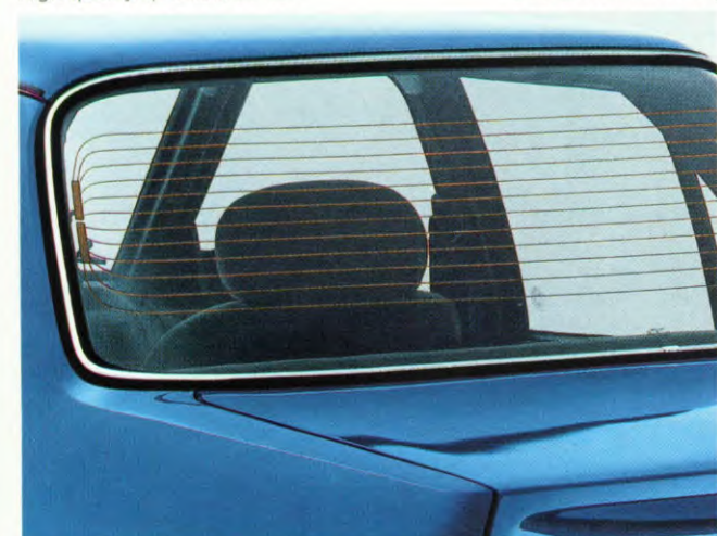
Radio-antenne in verwarmingselement (i.c.m. getint glas).
