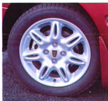
Alloy Wheel (7 Spoke) RRC 106040 MNH* Centre Cap DTC 10054 MNH Wheel Nut RRD 100310 Wheel Dimension 5.5J x 15 *Tyre change required
