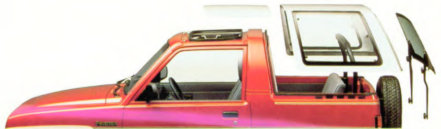
Sunroof is detachable. Resin top, backdoor window can be removed easily by unscrewing several bolts.
