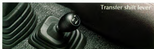
4L: Low-speed, 4-wheel drive For bad, muddy roads and steep grades
