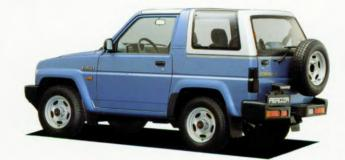
Sunroof is detachable. Resin top, backdoor window can be removed easily.
