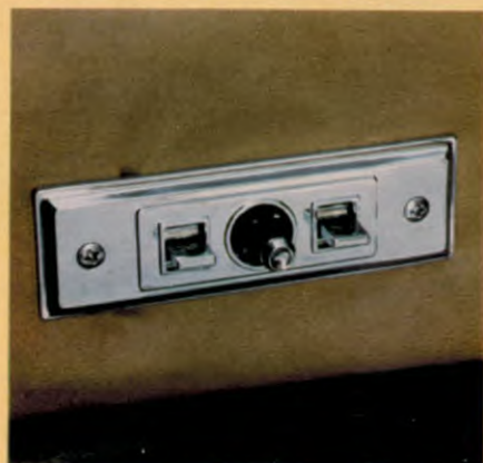
Power seats. Six-way adjustment lets you move the seat forward or backward, up or down, and tilt forward or back. Select the position that comforts best.
