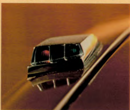
Fiber-optic lamp monitor. Tells when exterior lights are on or malfunctioning.
