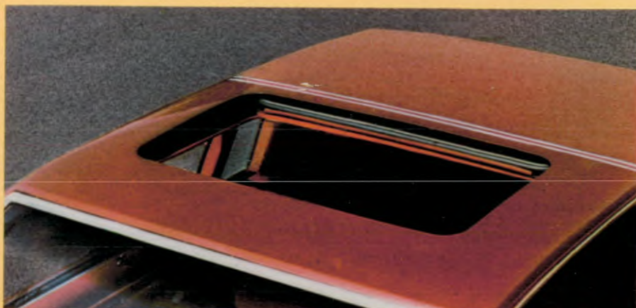
Electric sunroof. Panel slides into Cutlass roof to let the sunshine and air in. Reduces headroom slightly. Omega, Starfire offer removable sunroof.
