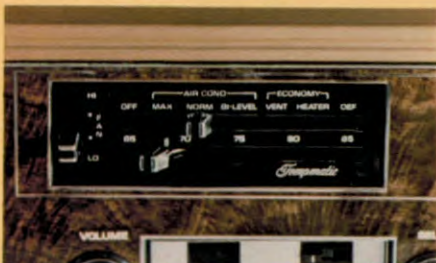
Tempmatic air conditioner. Cools, heats, dehumidifies and filters the air. Automatically maintains the temperature you select. Includes "economy" settings.
