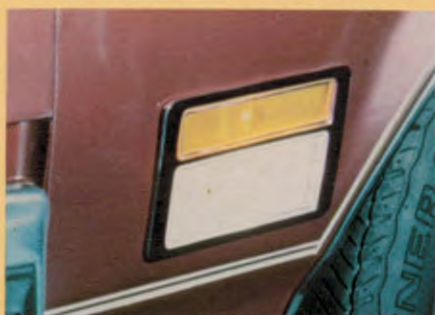
Cornering lamps. Controlled by your turn indicator whenever the headlamps are on. Directs light to the side in the direction you're turning. Cutlass only.
