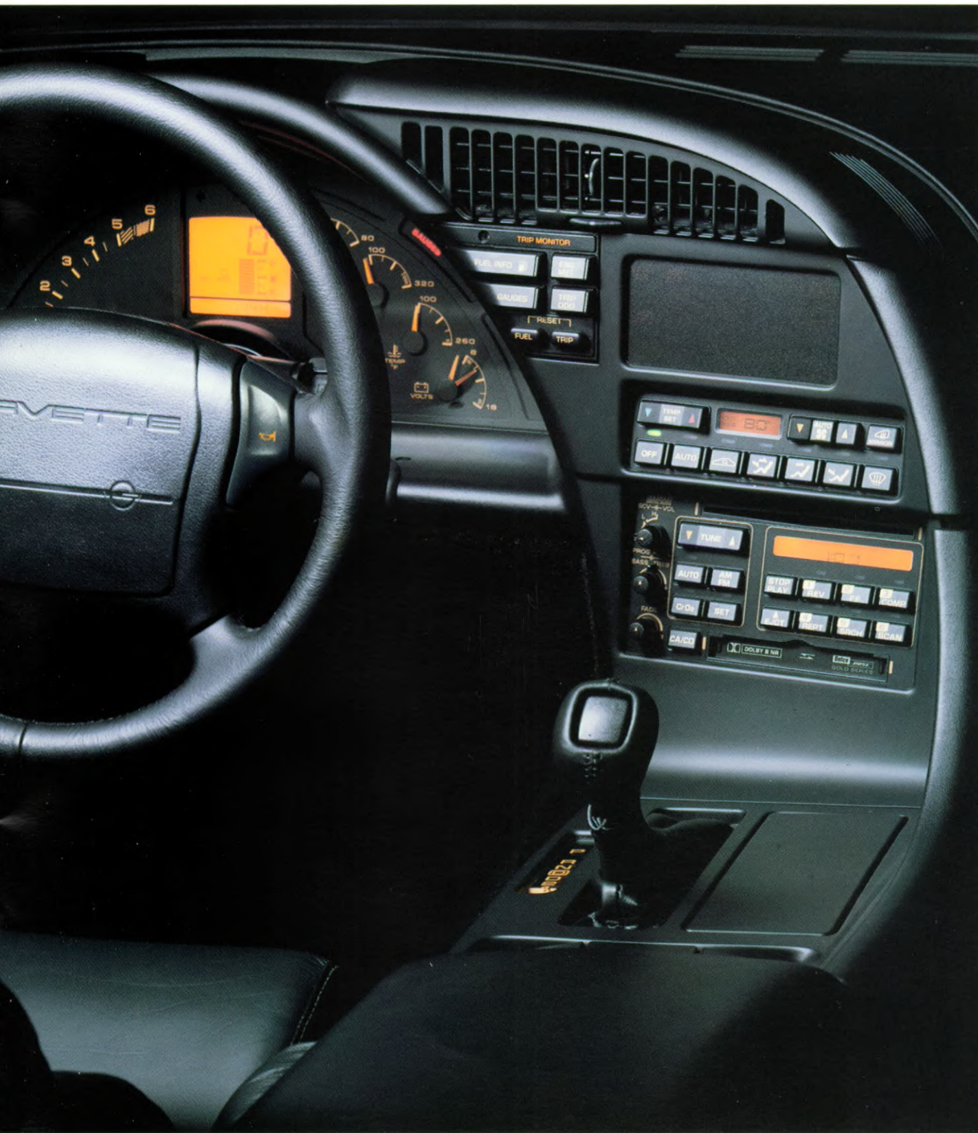
The Corvette instrument panel. Options shown include Delco/Bose stereo sound system with cassette tape player and compact disc player, and electronic-control air conditioning.
