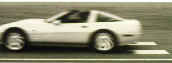
Polished steel pads simulate glare ice in a test of Corvette's new traction-control system.
