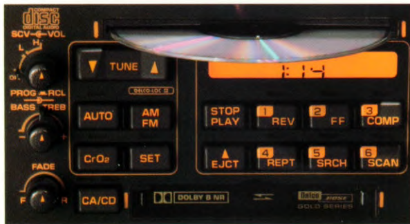
The sophisticated Delco/Bose Music System with integral cassette player and compact disc player is standard in ZR-1, optional in other models.
