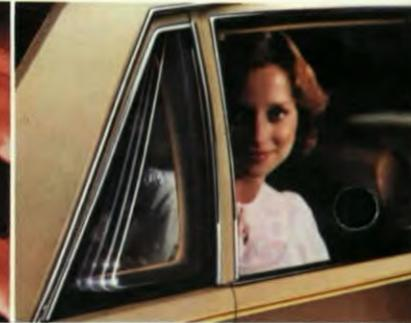
**Power vent windows.** Rear vent windows can be controlled in rear or from driver's seat. Included only with available front power windows on sedans and wagons.
