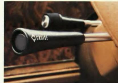
**Automatic speed control.** Maintains desired speed without touch of the accelerator. Disengages when brake pedal is depressed. Available with automatic transmission only.
