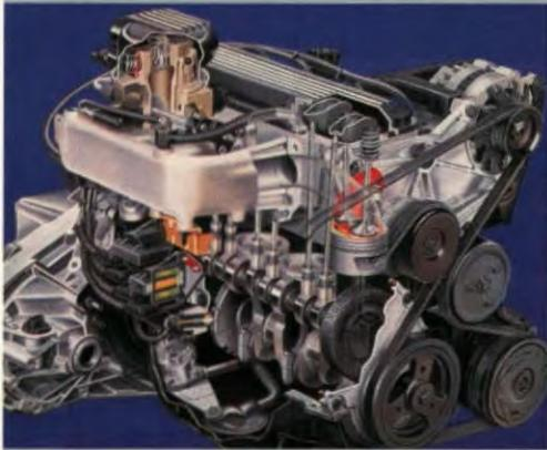
**Cavalier's 2.0-liter engine features increased horsepower and simplified Electronic Fuel Injection.**
