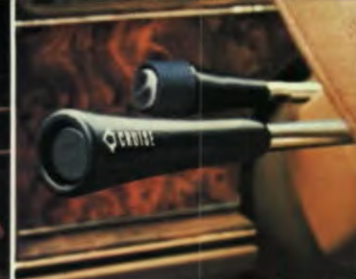
Automatic speed control. Maintains your set speed until the brake pedal is touched.
