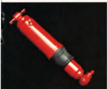
Inflatable rear shock absorbers. A great help when carrying extra-heavy loads.
