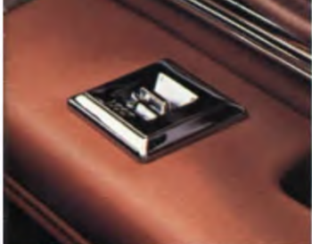
Power door lock system. Lock and unlock all doors from the driver's seat.
