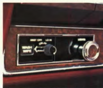
Intermittent windshield wiper system. Ideal for light rain or mist. Varies the wipe cycle.
