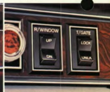
Power tailgate lock. Lock or unlock the tailgate from inside wagon. (Full-size wagon only.)
