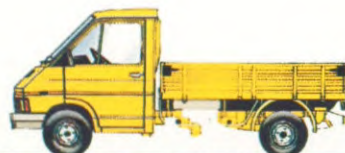
OPEN LAADBAK LANG ± 1000 KG LAADVERMOGEN
