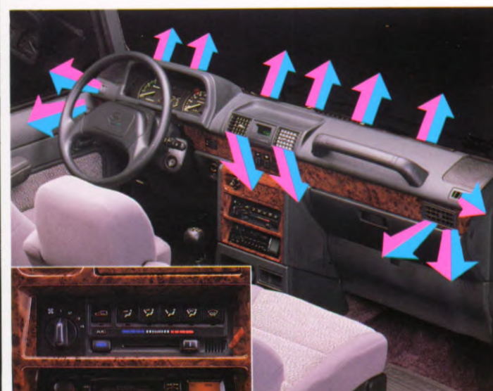
•The Korando is equipped with an upgraded 4,500Kcal/h climate control system.
