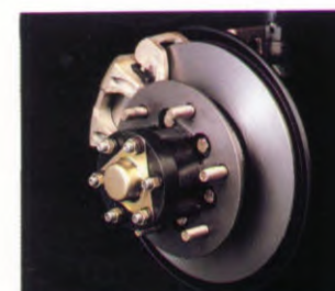
•Each Korando is also equipped with power, dual circuit, ventilated front disc and rear drum brakes, as well as antiheat, high durability brake pads.
