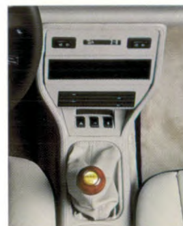
X21 Telefonkonsole für Bedienhandhörer. • X21 Alternatively, the Telephone Receiver can be fitted on the console to the front of the gear-shift lever.
