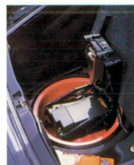
M612 The Philips Porty Transceiver Unit can also be housed in the wheel to utilise space.
