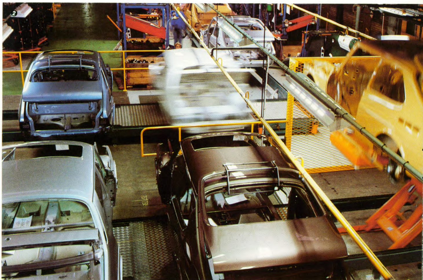
4. Robot welding of Saab car bodies.
