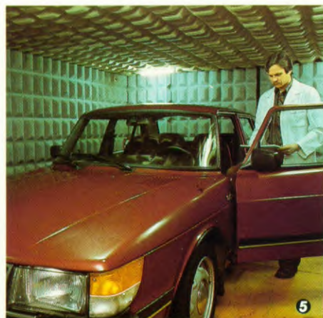
5. The sound laboratory aims for less vibration and less noise without heavy insulating materials. This reduces the car weight.
