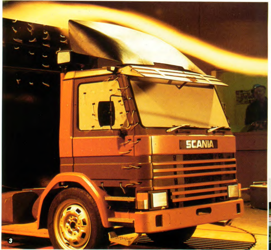
3. Wind tunnel testing of cabs on halfscale models.
