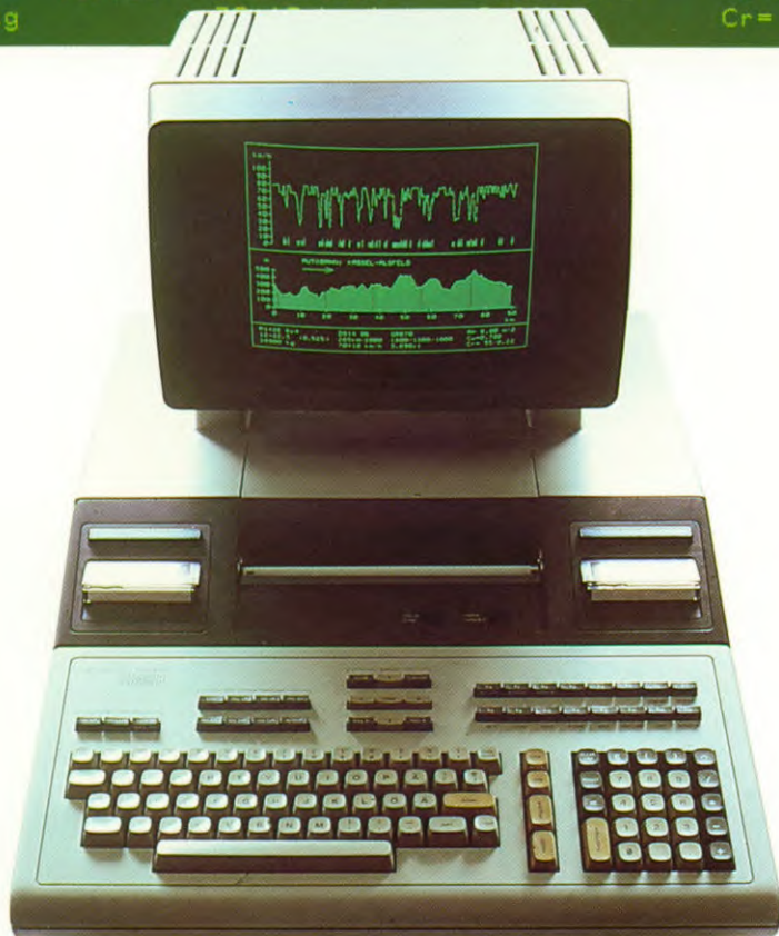
4. The STRASS computer program helps the truck designers to simulate driving on any road.
