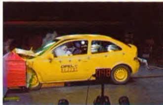
A: 40 406 - 271 40% offset deformable barrier, 56 km/h 40% Offset deformierbare Barriere, 56 km/h
