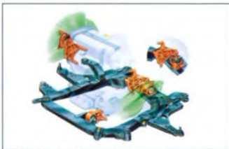
A: 40 175 - 115 Engine mountings: Neutral Torque Axis mounts (orange) Motoraufhängung; Lager (Orange) in der "Neutral Torque" Achse
