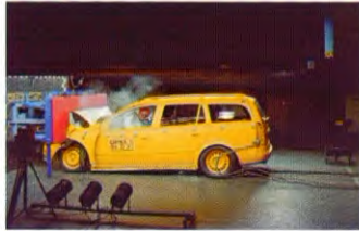
A: 40 409 - 275 0° Under-ride (Truck rear-impact), 40 km/h 0° Under-ride (LKW-Heckaufprall), 40 km/h
