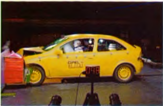
A: 40 405 - 270 40% offset deformable barrier, 56 km/h 40% Offset deformierbare Barriere, 56 km/h
