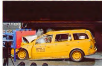
A: 40 410 - 276 0° Under-ride (Truck rear-impact), 40 km/h 0° Under-ride (LKW-Heckaufprall), 40 km/h
