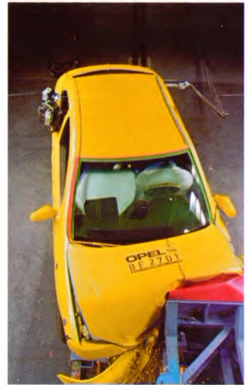
A: 40 407 - 273 40% offset deformable barrier, 56 km/h 40% Offset deformierbare Barriere, 56 km/h
