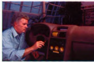
A: 40 498 - 152 Clay model of the instrument panel Modellieren der Armaturentafel
