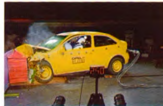
A: 40 404 - 272 40% offset deformable barrier, 56 km/h 40% Offset deformierbare Barriere, 56 km/h
