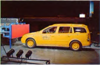
A: 40 408 - 274 0° Under-ride (Truck rear-impact), 40 km/h 0° Under-ride (LKW-Heckaufprall), 40 km/h
