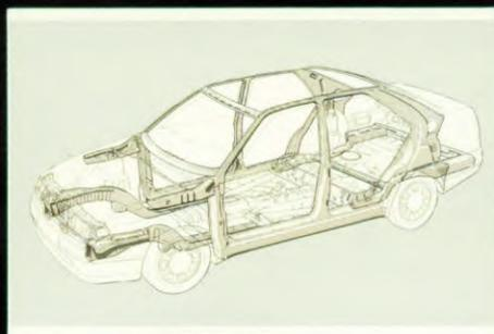
CHASSIS VAN DE TOLEDO ONDERWORPEN AAN EEN UITGEBREIDE ROESTPREVENTIE MET DE MODERNSTE BEHANDELINGSMETHODEN, WAARONDER EEN KATHODISCH DOMPELBAD, HET GEBRUIK VAN 'ZINCROMETAL' EN KUNSTOFBESCHERMING VAN FELSRANDEN, BODEM ETC... PROBLEEMLOOS KAN SEAT DAN OOK 6 JAAR ANTI-CORROSIE GARANTIE GEVEN. DIT IS DE SEAT TOLEDO, EEN TOTAALCONCEPT, DAT ZICH NIET BEPERKT TOT HET BRENGEN VAN RIJPLEZIER OP HET HOOGSTE NIVEAU, MAAR OOK KLAAR IS OM TE BEANTWOORDEN AAN DE EISEN VAN DE TOEKOMST.
