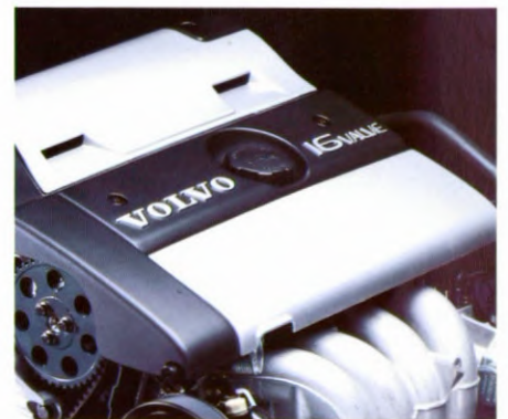
4 cilinder 16V, in 1.8 of 2.0 liter leverbaar.
