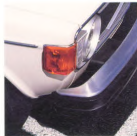
1973 Energie absorberende bumpers
