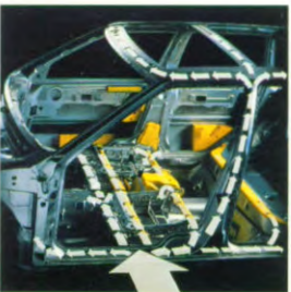
1991 SIPS Side Impact Protection System
