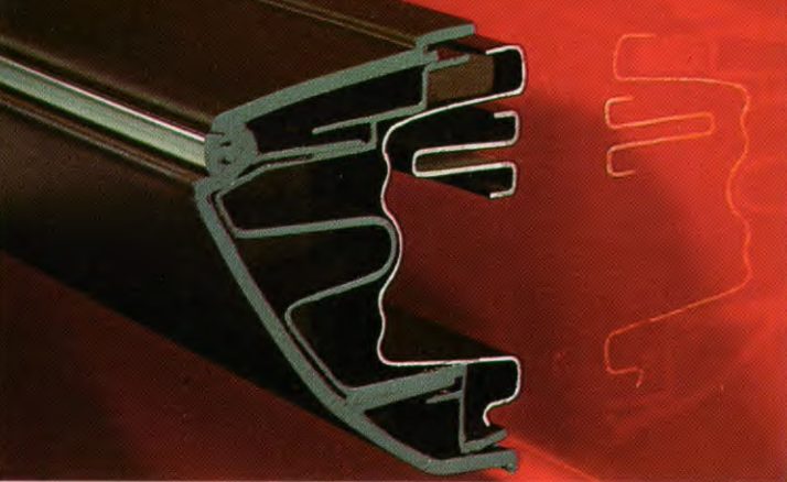
Two-piece composite bumpers are used on the Scirocco. Inside, a robust steel girder; outside, a tough plastic facing that absorbs minor bumps when parking.
