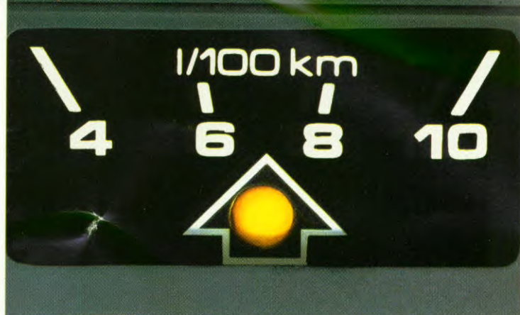
The gear-shift and consumption indicator (not on models with 40 kW engine). It reminds the driver (of a manual-gearbox car) to change to a higher gear in good time, the second part shows him, once top gear has been selected, just how much fuel the car is consuming.
