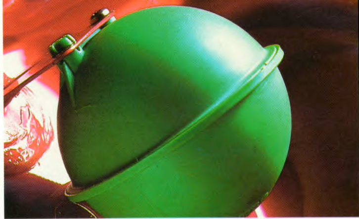
The carburettor must be influenced for smooth running when the engine is still cold. This is done, for instance, by means of this vacuum can.
