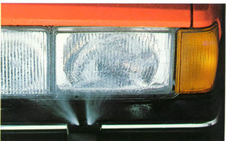
Standard equipment on the Scirocco GT: the headlight cleaning system. It uses water at high pressure for clean headlights, better vision and greater safety.
