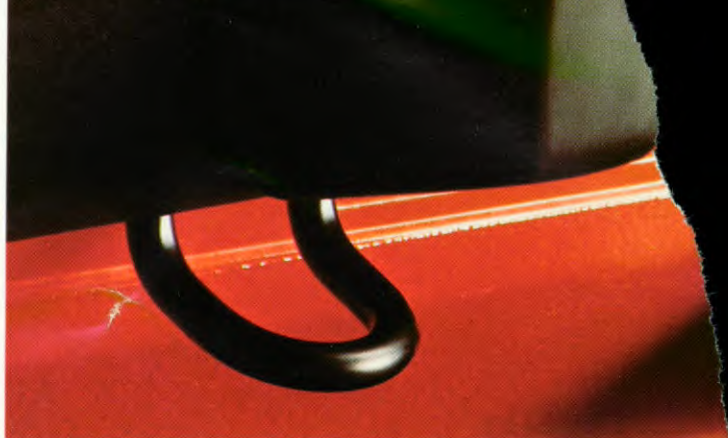
The Scirocco has a substantial towing eye at the front, directly above the integral front spoiler. A towrope can easily be attached in an emergency.
