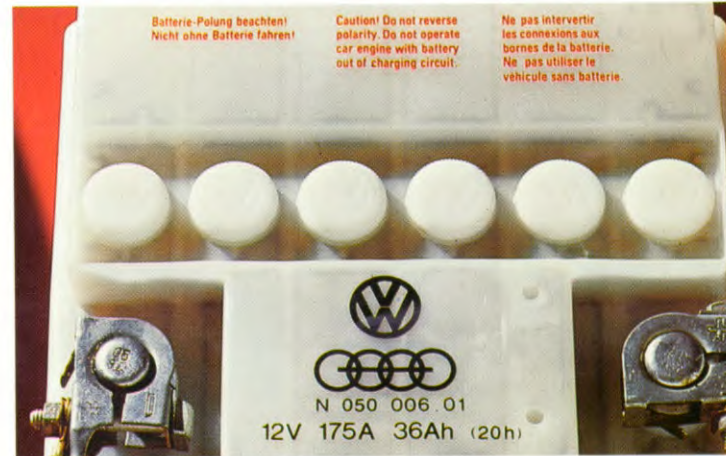
To simplify maintenance, all Scirocco models are equipped with a battery that needs no routine attention, apart from checking when the car is taken in at the specified servicing intervals.
