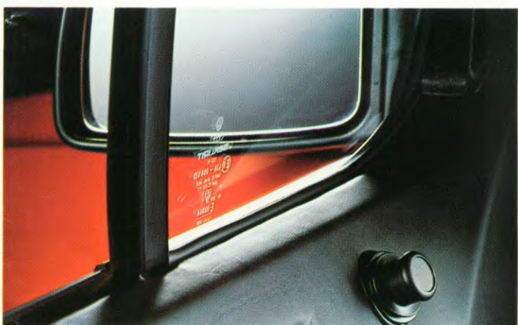
This is an important control: it alters the door mirror setting on the Scirocco GT from the inside.
