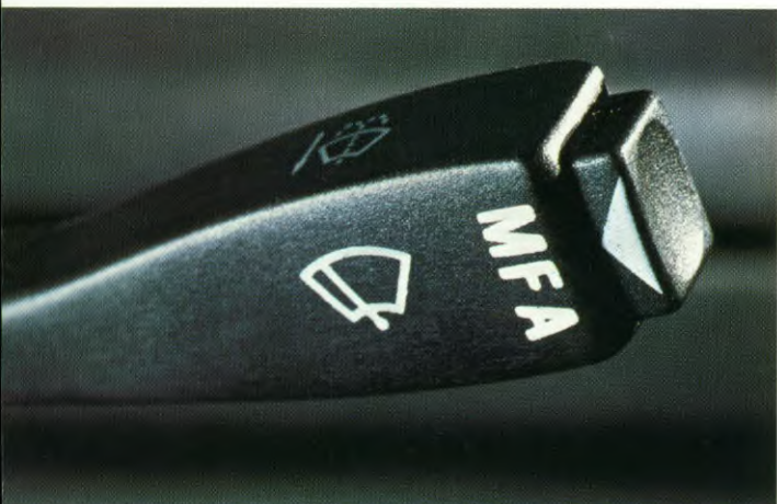
When the button is pressed, the digital display reads out real time, journey time, journey distance, average speed, average fuel consumption, oil temperature and outside temperature. (Optional extra for cars with 82 kW.)
