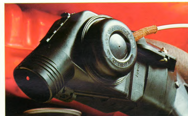
A thermostat in the air cleaner housing reacts to outside air temperature and controls intake air preheating automatically.
